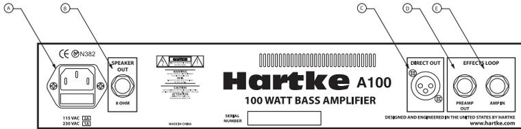
**A. AC Power Inlet** - Use the supplied grounded AC power cord to connect your A Series amplifier to mains power. This cord comes supplied with the appropriate plug for your geographic area. CAUTION: Do not use an adapter to defeat the third grounding pin on this plug or severe electric shock may result!
