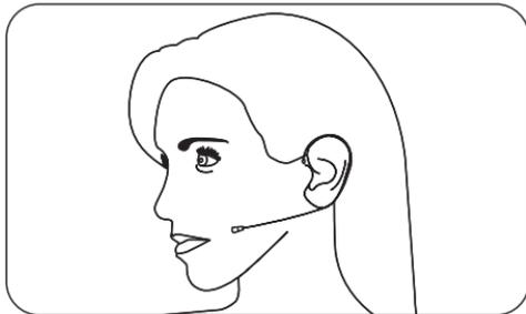
Position the DE50x microphone element about 0.25" – 1" behind the corner of your mouth. Since the DE50x is an omnidirectional capsule, the end of the microphone does not need to be facing your mouth. To avoid breath noise and p-pops, do not place the microphone directly in front of your mouth.
