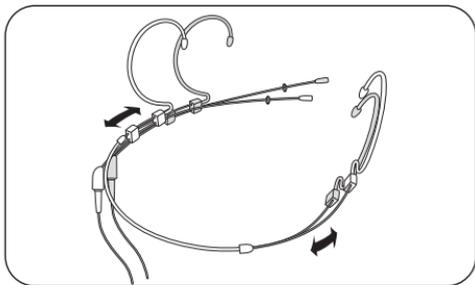
The headset can be re-sized by sliding the ear hooks to fit snug around your head. If the DE50x is loose and will not stay in place, slide the ear hook wires back for a tighter fit.
