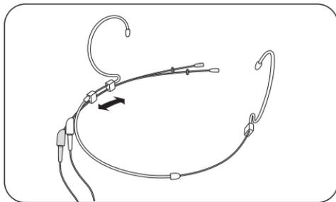
Adjust the microphone position by holding the left ear hook wire and slide the boom forward or back. For optimum performance the microphone should be close to the skin and towards the corner of the mouth, approximately a half inch away.
