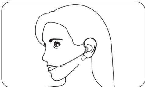
Position the SE50x microphone element about 0.25" – 1" behind the corner of your mouth. Since the SE50x is an omnidirectional capsule, the end of the microphone does not need to be facing your mouth.
